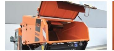
The construction of the sweeper's container with a wide rear door opening enables unloading of waste into municipal containers.
