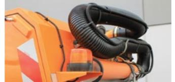
The sweeper is equipped with a manual suction hose for cleaning garbage disposal cans, sewer holes and areas that MUVO cannot reach with its front brushes.
